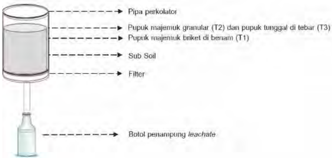
Gambar 1. Desain pipa perkolator, packing sampel tanah, penempatan pupuk, dan botol penampung hara tercuci Figure 1. Design of percolator tube, packing of soil sample, placing of fertilizers, and container for collecting leachate.
