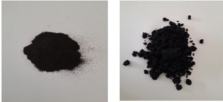
Figure 1. Dry biochar (a), biochar soaked in water for 7 days Gambar 1. Biochar kering (a), Biochar yg direndam air 7 hari
